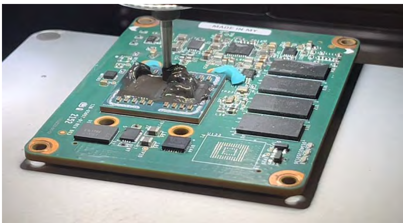
Polished IC backside (720 um thickness reduction)
